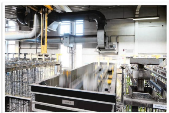
A rack elevator enables the separation of the loading and chrome plating zones (ghost production) /22/
